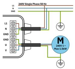
The terminal block inside the controller is clearly labelled. Incorrect wiring will destroy the electronic circuit board.
